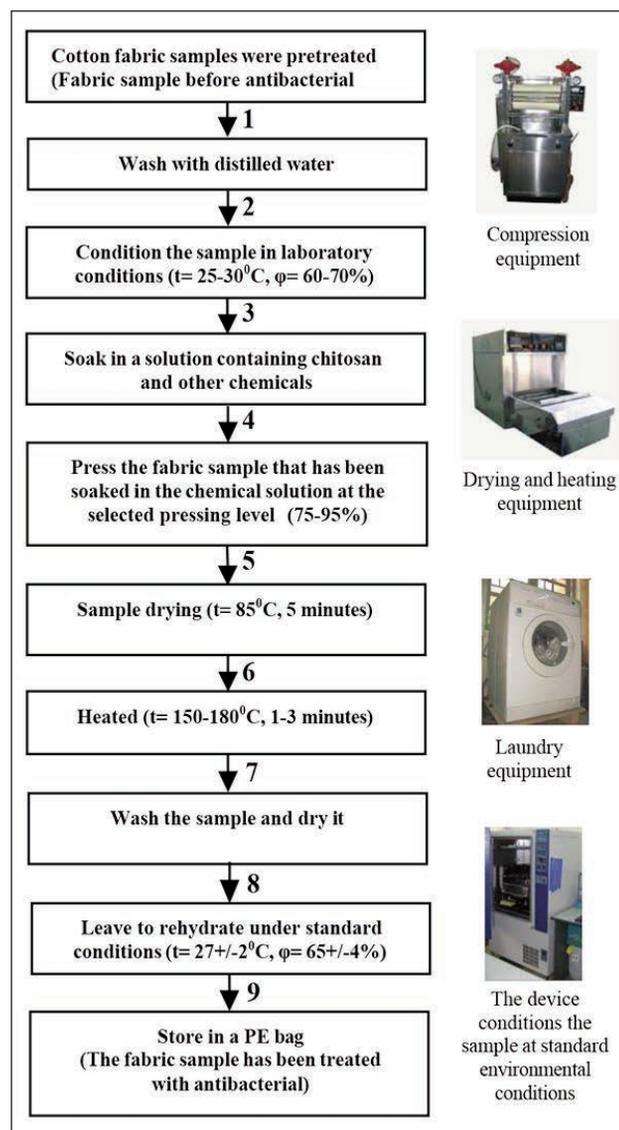
Fig. 1. Process of attaching chitosan to cotton fabric
